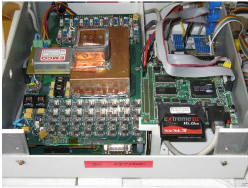
Fig. 3. The SIDERALE payload. In the foreground on the left, the ADC board stacked on the FPGA-based board, the pre-amp shield, and the detector assembly (16 pixels CZT) on top of it; on the right, the single board computer and the 16 MB Flash memory.
