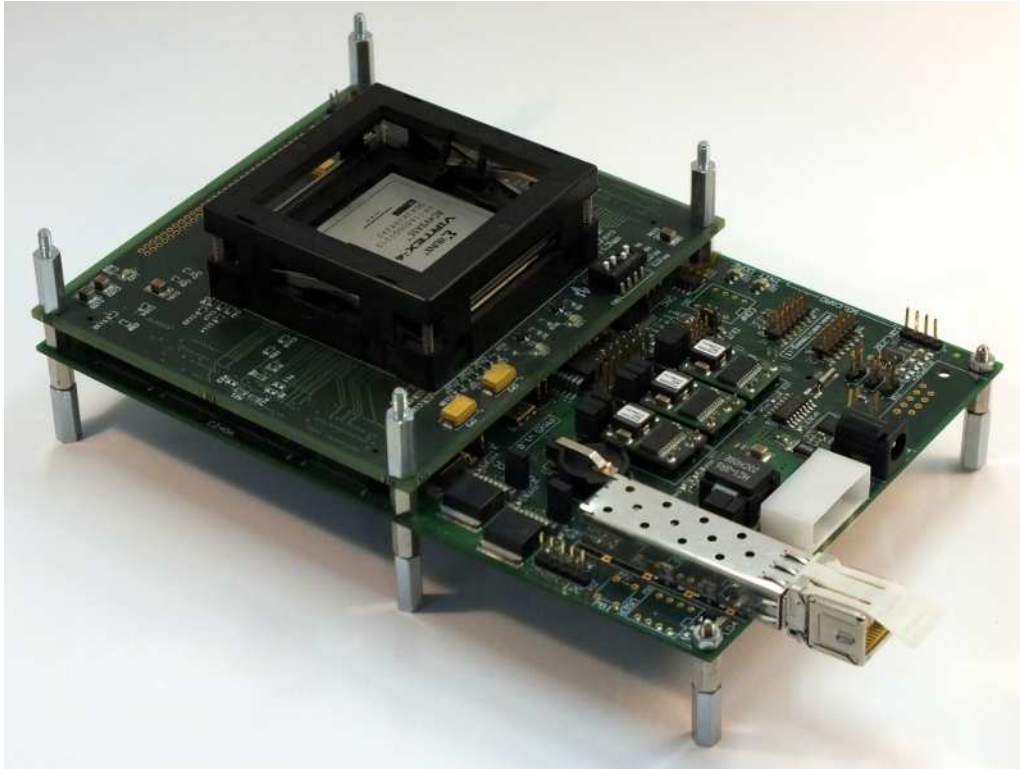
Fig. 1. FLIPPER Hardware platform. The picture shows the control board and the DUT board with a Xilinx XC4VSX55 stacked on it.
